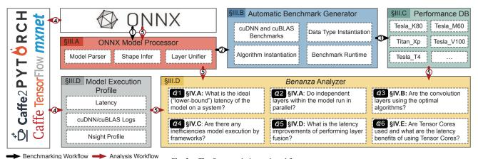
Fig. 2. The Benanza design and workflow.
