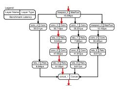
Fig. 5. The first parallel module of Inception-v1 in Figure 8 visualized by the *Benanza* Analyzer. The layers are annotated with the name, type, and latency used for the "lower-bound" calculation. The critical path used in the parallel mode is highlighted in red.
