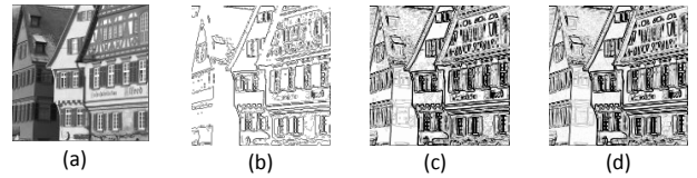
Figure 7. Progressive precision results for edge detection: (a) input image; output image after (b) 4, (c) 32, and (d) 256 clock cycles.
